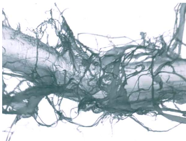
Refined fiber and fibril releasing
