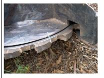
Motor saws, feller bunchers and harvesters consume and waste wood to saw the trees. The harvester design may also result in a high stub cut (about 20 cm), which means losing wood that turns into sawdust in the cutting area, as well as losing wood due to the remaining stub height.
